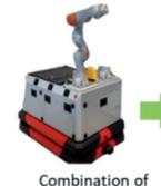
Combination of AGV+ Robot Arm
