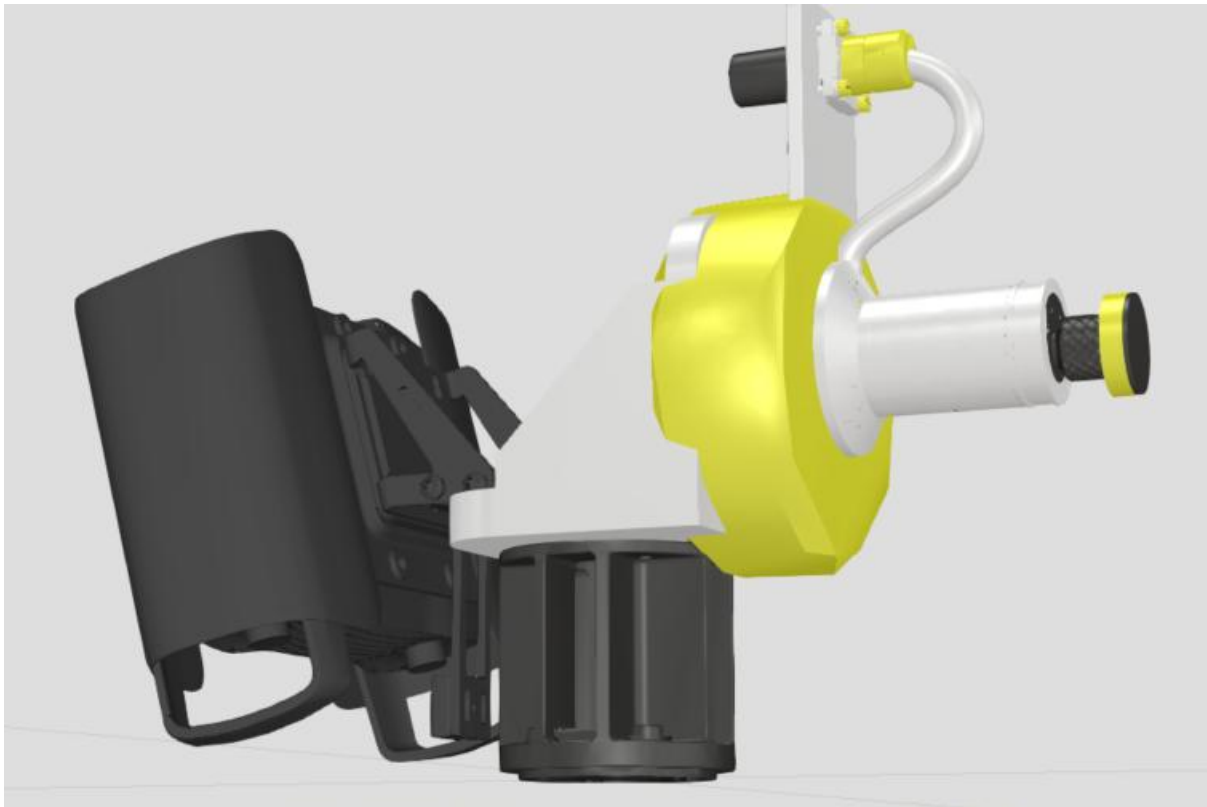
Figure 23: Mobile Polishing Robot End Effector Design.
