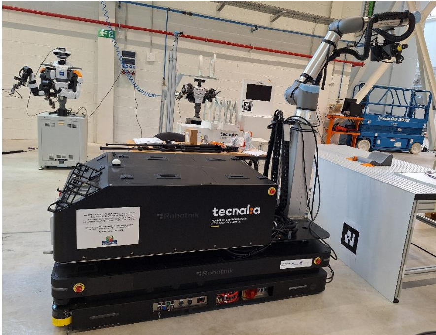
Figure 4: Actual current mobile manipulator with Zivid and Mirka end-effector.
