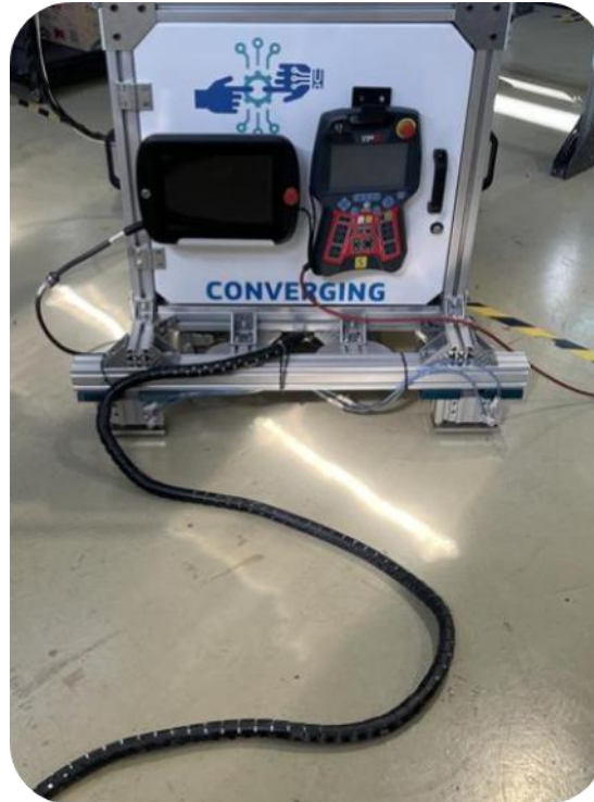
Figure 35: Cable management tube for all cables of cart.
