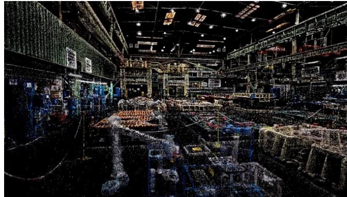
Figure 13: Reconstruction through Gaussian Splatting. Point cloud image to show that it is a 3D image.
