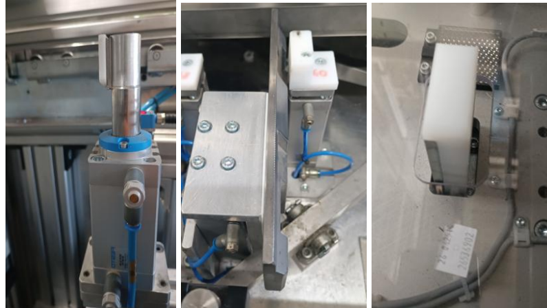
Figure 26: Hob centering mechanisms available at ELUX.
