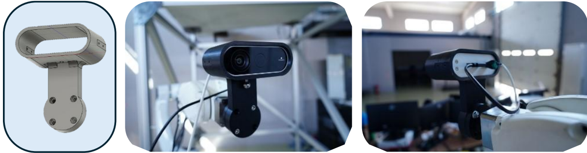
Figure 37: Protective mount design and final installation on robot.
