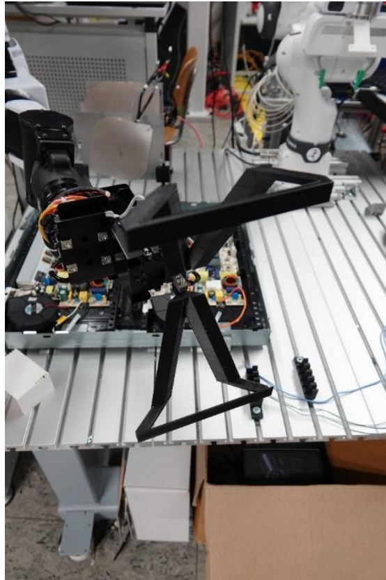
Figure 22: Detailed view of coil grasping fingers.
