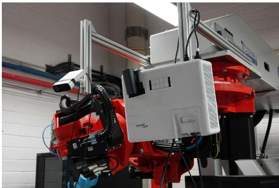
Figure 23: Detailed view of projector and cameras on the mounting system.
