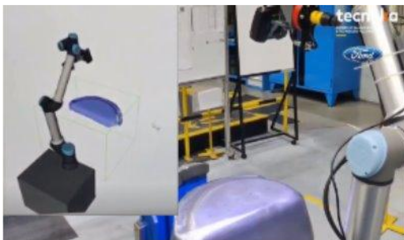
Figure 5 PAM module performing the scan of a die.
