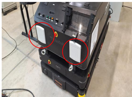
Figure 6: Newly installed fans on the mobile manipulator for cooling.
